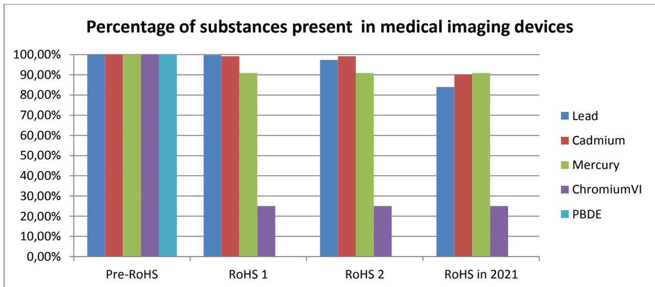
**Fig 1:** graphical representation of content of RoHS 6 substances in medical imaging devices before and after RoHS I and RoHS II.
