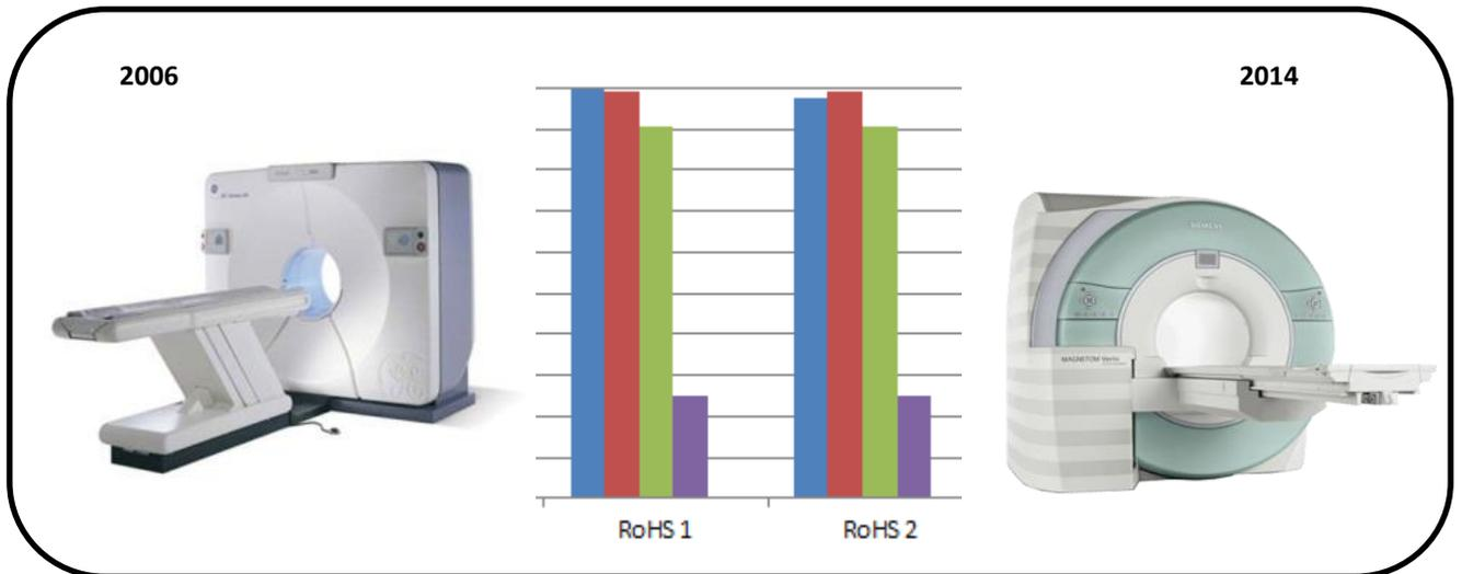
**Fig 2:** Difference between medical devices before and after RoHS II. Only lead is slightly affected by RoHS II (same color code of Fig 1).
