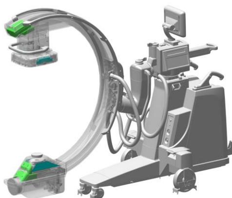
The lead counterweights need to be sizable to counter balance the weight of the C-arm and cables inside the C-arm. Due to limited space near the x-ray tube and detector the shapes have been made to fit unique shapes to make use of all available space.
