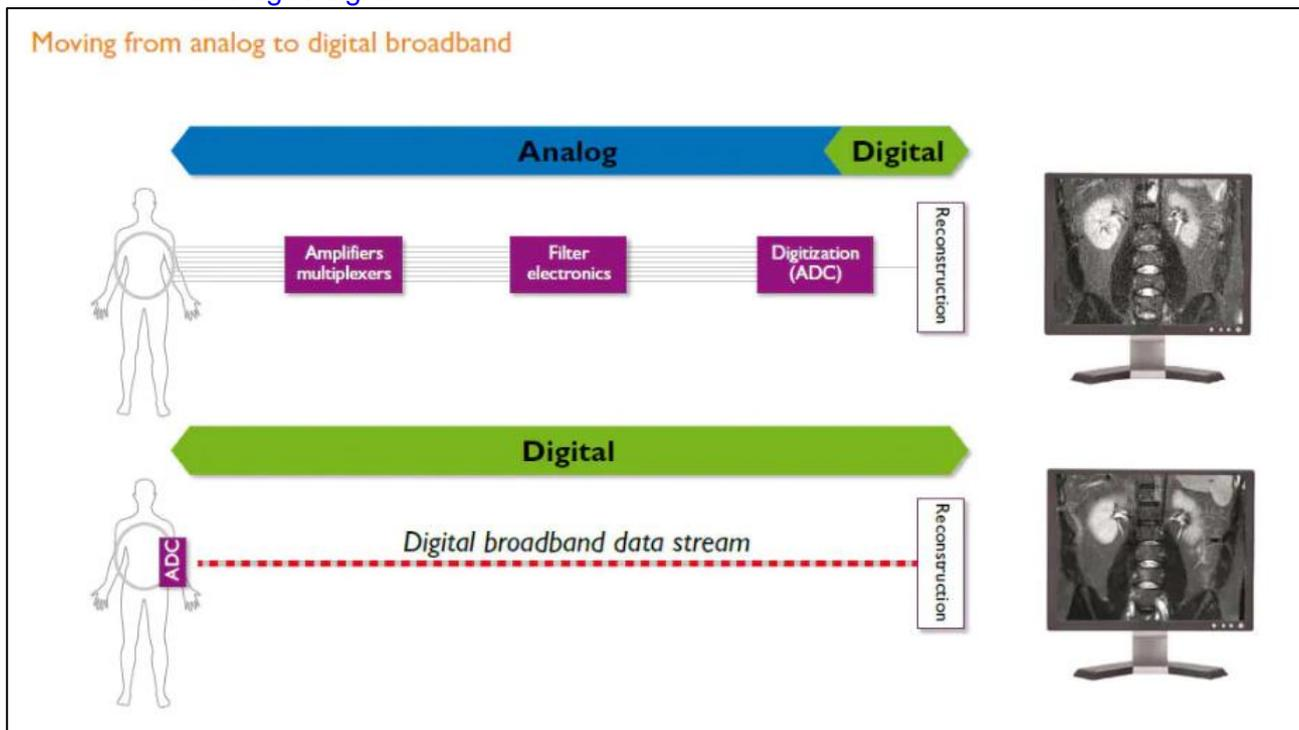
*The RF-receiver coil is the first element of a complex electronic chain by which the MR signal is amplified, digitized, decoded, and transferred to the main computer system for processing into the final MR image.*
