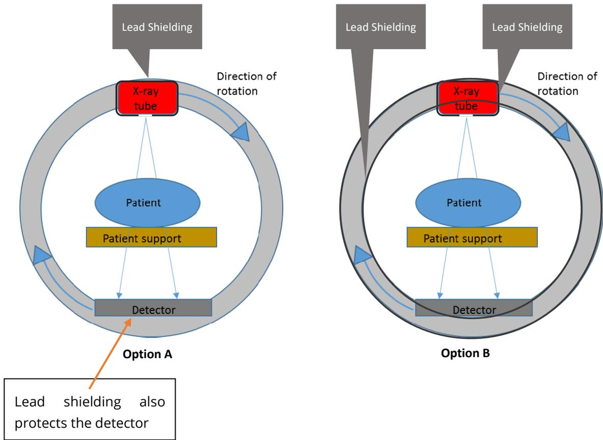
**Figure 2 Diagram of Option A and Option B Shielding**
