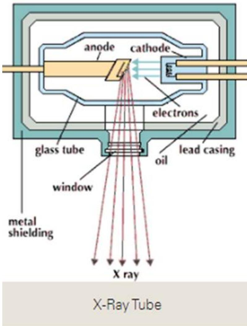
Figure 1 Conventional X-Ray Tube Housing
