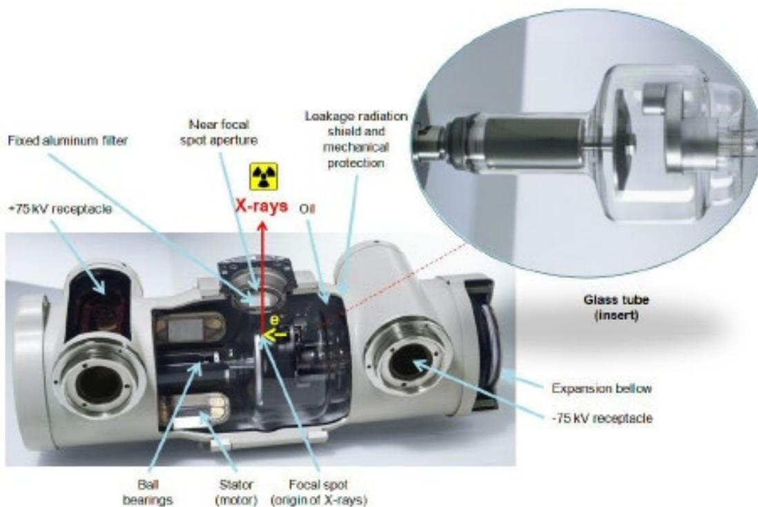
**Figure 3 Conventional X-Ray Tube Housing Assembly with ball bearing**
