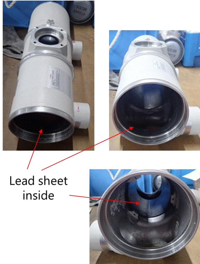
Figure 1. Lead sheet shielding used inside an X-ray tube
