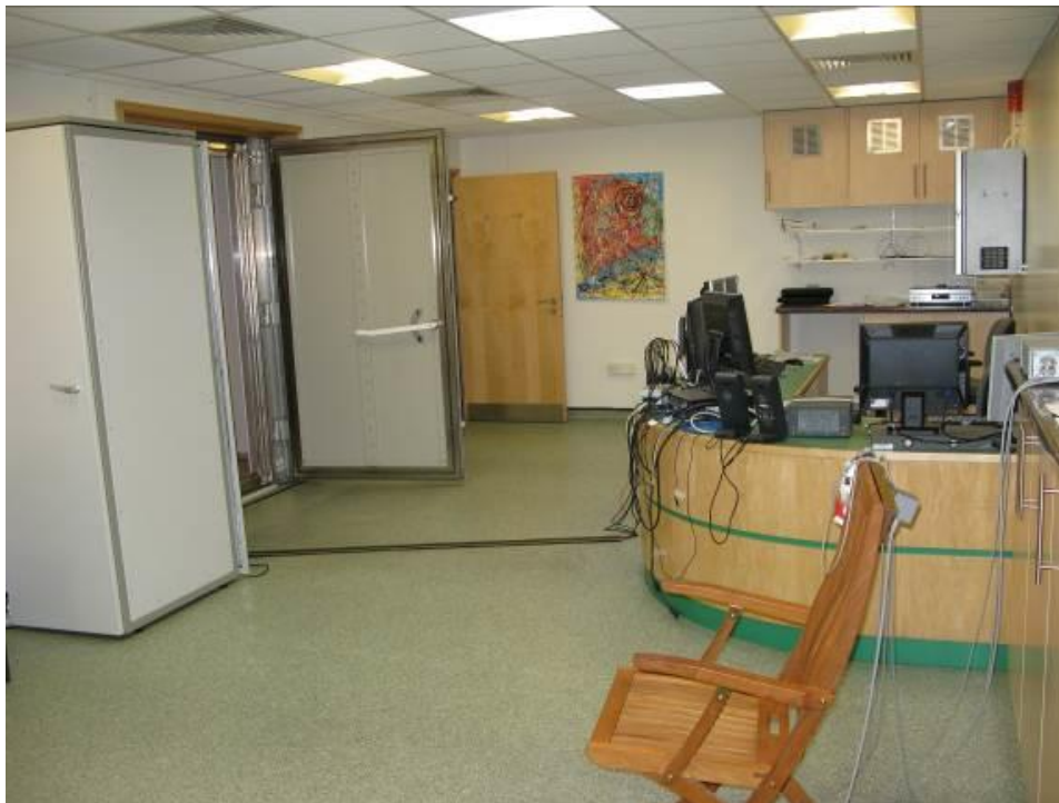
A view from operator's area. The open door metal-framed door is the entrance to the magnetically shielded room.
